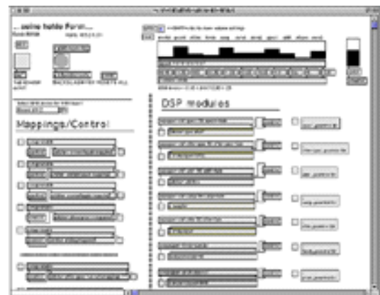
Figure 2: The MAX/MSP program for "Seine hohle Form", designed by Butch Rovon, is a musical synthesis environment that provides many control parameters, addressing a number of custom-built DSP modules that include granular sampling/synthesis, additive synthesis, spectral filtering, etc. Control of the musical score to "Seine hohle Form" is accomplished through a cue list that enables/disables various EyeCon movement analysis parameters (see Figure 3), mapping and DSP modules to be implemented centrally.
