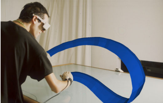
Figure 1: The path of the hand in space is converted to a geometric stroke that floats in space, as shown in this composite image.
