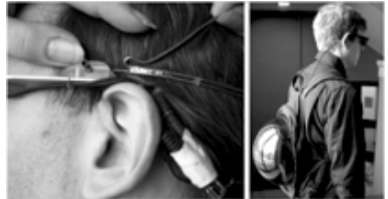
Figure 3: (a) A close-up of the proprietary security screws and copper comfort bands.
