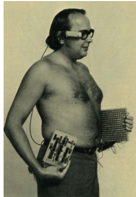
Figure 5: Sensory substitution device for haptic vision by Bach-y-Rita (Image taken from [1]).
